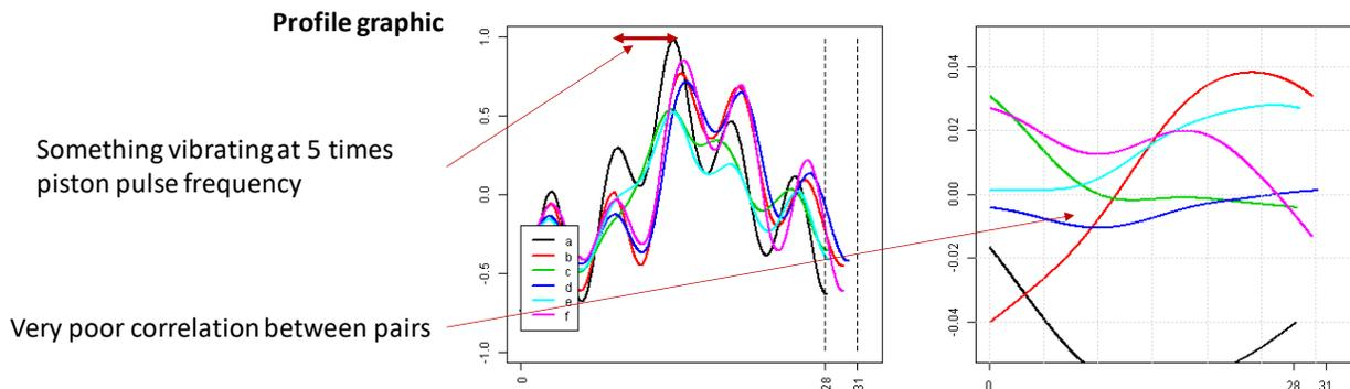
Fig. 5. The Profile graphic for the subject engine at idle.
