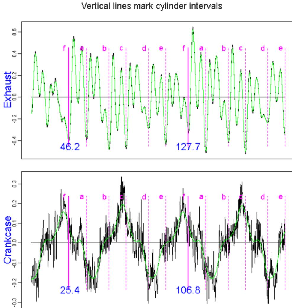
Fig. 1: A signature of a V6 engine running at 1473 rpm with the exhaust sensor sampling exhaust pressure at the end of the tailpipe and the crankcase vapor pressures from the oil dipstick tube.
