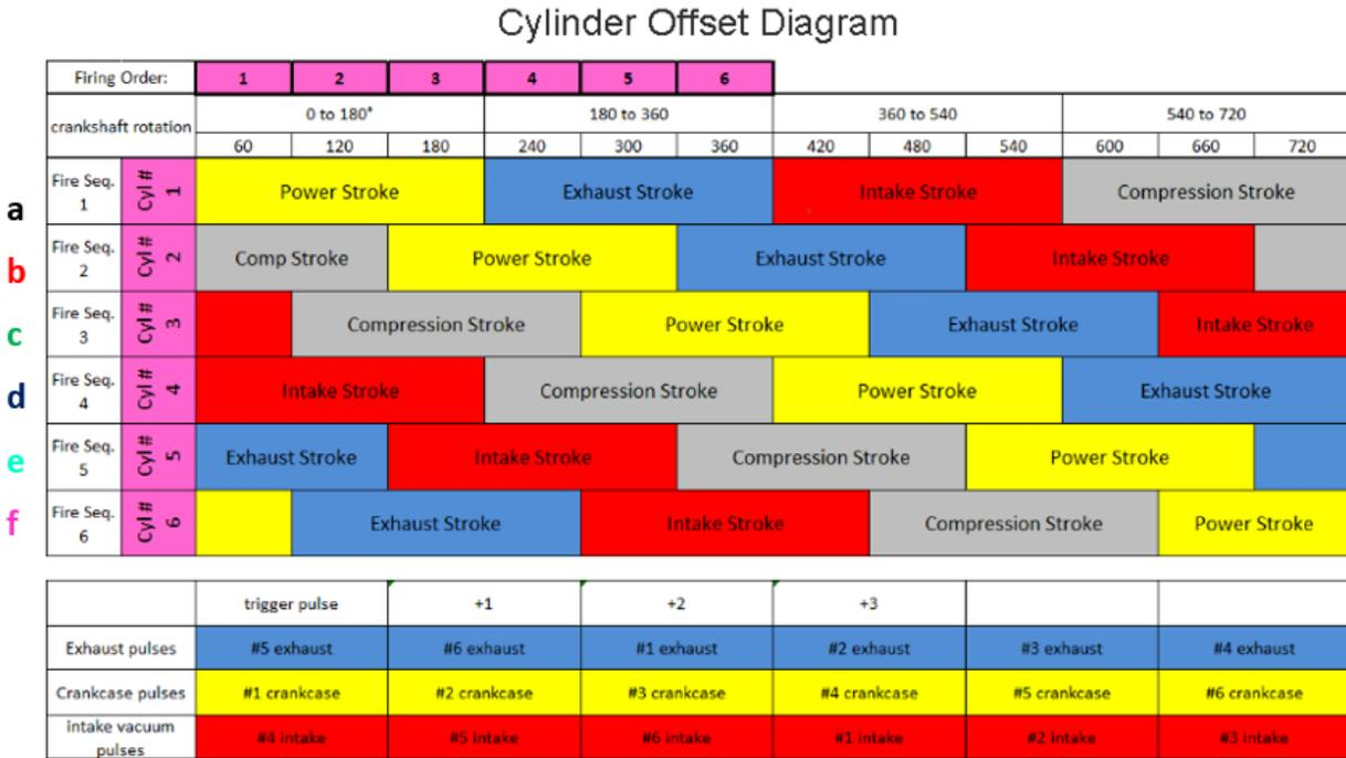
Fig. 11. Cylinder Offset Diagram for the subject engine.
