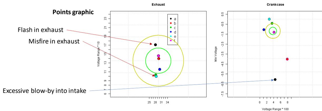
Fig. 4. The Points graphic for the subject engine at idle.
