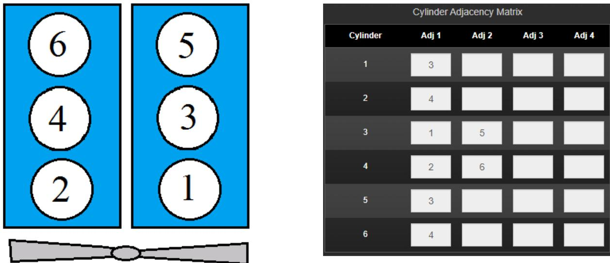
Fig. 10. Engine Block Diagram and Connectivity table for subject engine.
