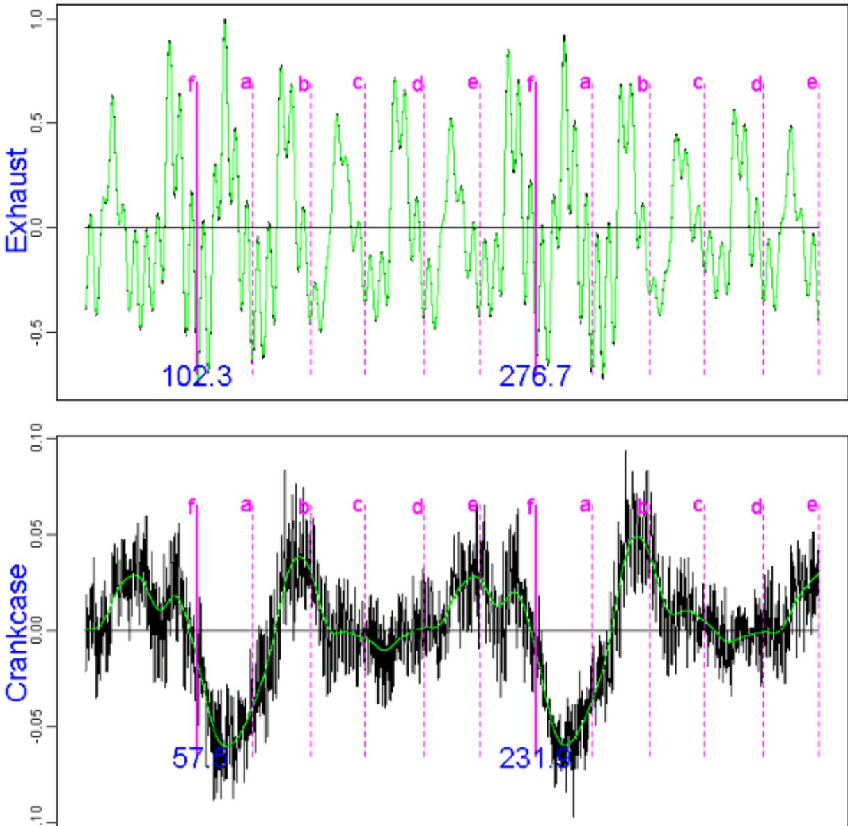
Fig. 3. Signature for 20200402-0001. Engine is a 3.0L 3100 GM LFW V6) at idle. The time markers (ms) define the rpm =  $30000 * \text{NumberStrokes} / (276.7 - 102.3) = 688 \text{ rpm}$
