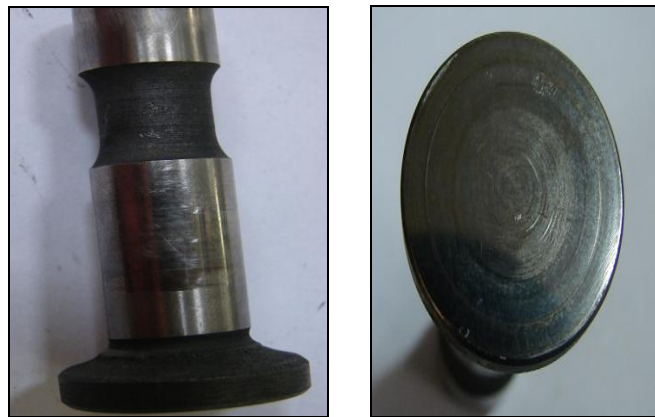
Fig 6 Wear Marks on outer diameter and bottom face of the Valve tappet.
