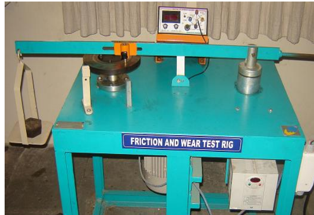
Fig 3 Pin on Disc Wear Test Rig
