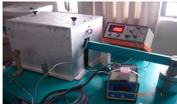
Fig 4 Pin on Disc Wear Test Rig with heating chamber
