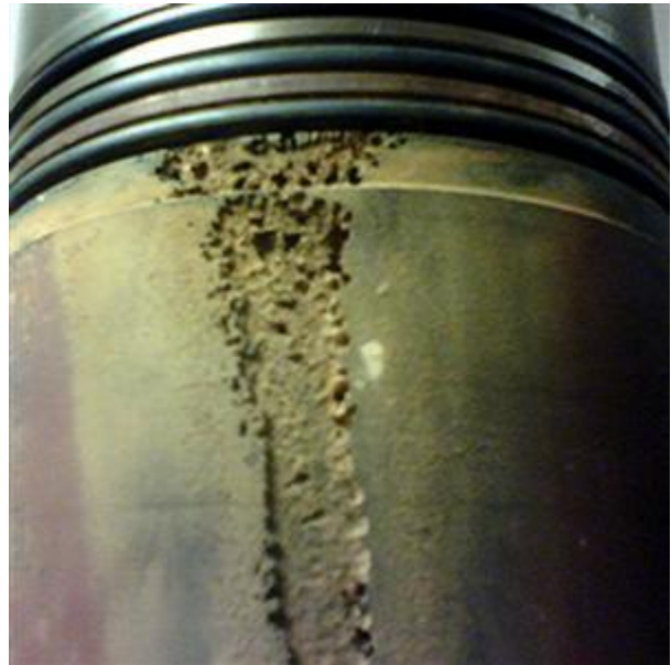
A diesel cylinder liner showing the effects of cavitation erosion.
